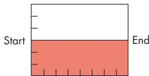
The Double Acting Actuator has a constant output torque throughout travel from start to end, clockwise or counterclockwise rotation
