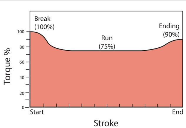
**PNEUMATIC ACTUATOR DOUBLE ACTING TORQUE CURVE**
