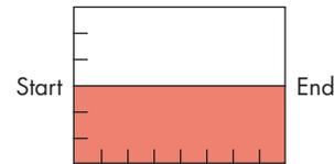
Electric Actuators have a constant output torque throughout travel from start to end, clockwise or counter-clockwise rotation.
