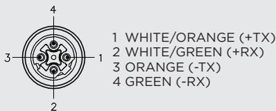
Terminate directly onto the Servo NXT EtherNet/IP TX+/TX- & RX+/RX- terminal points.
