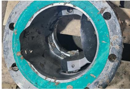
**CHALLENGE:** Typical valves show extreme solids buildup or accelerated erosion after only a few months of service in harsh pulp & paper applications.
