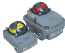
SERIES 5A / 5B VALVE STATUS MONITOR NEC CLASS I DIV 1 A,B,C,D CLASS II/III DIV 1 E,F,G ATEX/IECEx G ZONE 0 IIC
