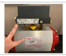
2.6 Insert the pneumatic fittings on the positioner and actuator before inserting tubing into the outputs of the positioner to the inputs of the actuator.
