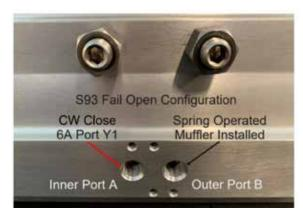
Insert the pneumatic fittings on the positioner port Y1 and actuator inner port A before inserting tubing between these two pneumatic fittings.
