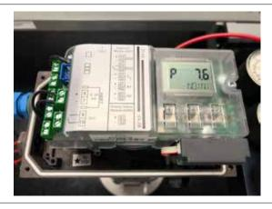
73.2.2 Press the Menu Button for >5 seconds to enter into Configuration mode.
