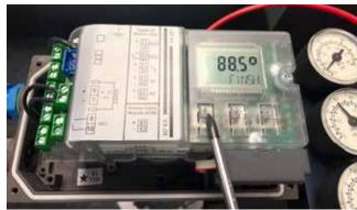
3.1.13 Press the Menu Button for 5 seconds. The device will now be in 'MANUAL' mode.
