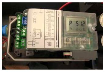
3.1.11.1 Adjust the gray friction clutch adjustment wheel until the screen displays a "6" in the top right hand corner.
