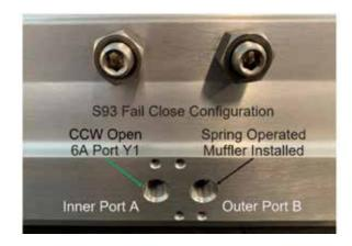
Only the inner port A will be connected to the 6A positioner at port Y1. The piston rack to pinion orientation determines the spring fail position, see S92/S93 IOM for details.
