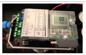
3.1.14 Use the  $\overline{\nabla}$  or  $\underline{\triangle}$  buttons to manually close or open the valve to ensure that the desired travel limits are being attained.
