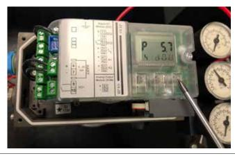
3.1.12 Upon successful completion of calibration, the status line will display "FINISH".
