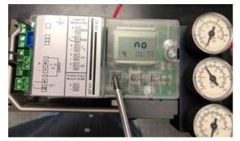
3.1.10 Hold down the Up Button \(\Delta\) until calibration begins (>5 seconds), then release. The device will now progress through 5 "RUNS", completing a series of checks. For more information on the calibration, please refer to the product manual.
