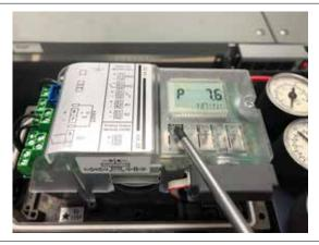
3.1.7 Once in Configuration mode parameter is displayed in the bottom left hand corner of the positioner screen. Use the Up Button ⚠ to scroll through the available options in ascending order and the Down Button ∇ to scroll through the available options in descending order. Press the Menu Button to scroll through the parameters in ascending order.
