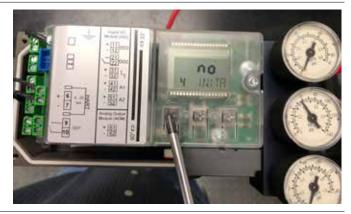
3.2.6 Hold down the Up Button 🛆 until calibration begins (>5 seconds), then release. The device will now progress through 5 "RUNS", completing a series of checks. For more information on the calibration, please refer to the product manual.
