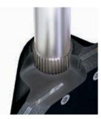
the splined stem from the disc. The Tri Lok connection allows axial movement of the disc independent of the stem. Therefore, the seal ring and seat remain in position, unaffected by temperature fluctuations and pressure effects on the stem. The splined connection offers
