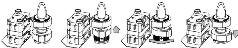
4. Release the cam and allow the locking spring to re-engage the cam with the fixed cam holder.
