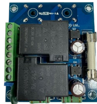
Figura 32: 24V CA/CC On/Off Tablero de Control.
