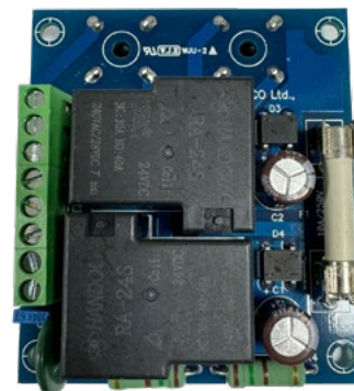
Figura 31: 24V CA/CC On/Off Tablero de Control.
