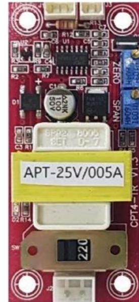
**Figura 32:** 24V CA/CC On/Off Tablero de Control.
