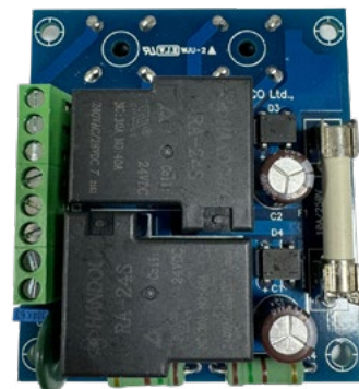
Figura 31: 24V CA/CC On/Off Tablero de Control.
