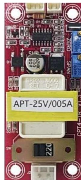
**Figura 31:** 24V CA/CC On/Off Placa de Controle.
