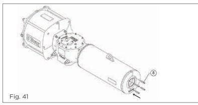
9. Insert the damper assembly into the spring module, locating the flange through the studs. Press the flange to mate the inside face on the flange to the spring module's end cap and secure the assembly with the spring washers and nuts. Tighten the nuts, refer to below table for torque values.
