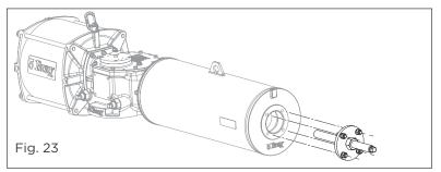
5. Tighten the nuts with spring washers; refer to Table 10.4 for tightening torque for the nut size.
