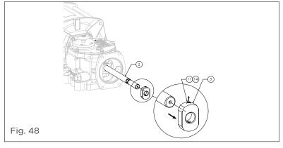
4. Unscrew the tubular cover (6) off the PST&LD module.
