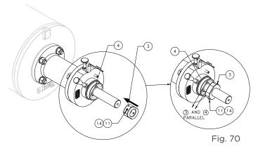
15. Fit back the tubular cover, threading it fully over the sleeve threads and the O-ring
