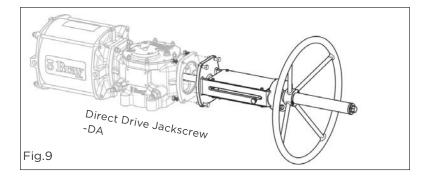
7. Slide the assembly to locate and mate the flanges. Use the hardware supplied in the kit to fasten the assembly to the Torque Module flange.
