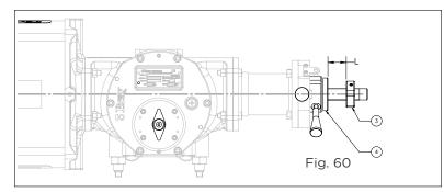
4. Return the actuator to the CW end. Turn the locknut a bit clockwise to align the locknut's flat faces to the sleeve's flat sides, so that the sleeve's profile will not interfere with the locknut when the extension rod moves inwards. Lock the set screws to secure the position of the locknut.
