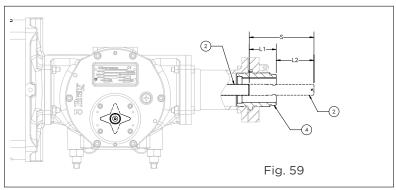
Loosen the locknut (3) by first slackening the set screws (11). Set the distance "L" between the index sleeve's outer face and the inner face of the locknut per the below table.
