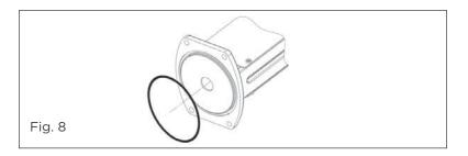
6. Back off the jackscrew fully in the assembly and carefully slide the mounting flange of the jackscrew assembly on the extension rod. Take care in locating the bushing and the flange seal on the extension rod.
