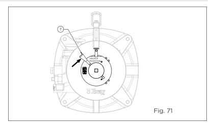
2. Unscrew and remove the tubular cover. Thread in the lock nut (3) on the extension rod threads with the inside face of locknut right up to the face of the index sleeve (4). Turn the nut a bit counterclockwise, to align the flat sides on the lock nut with the flats in the sleeve, so that the nut will enter the sleeve without any interference when the extension rod (2) moves inwards.
