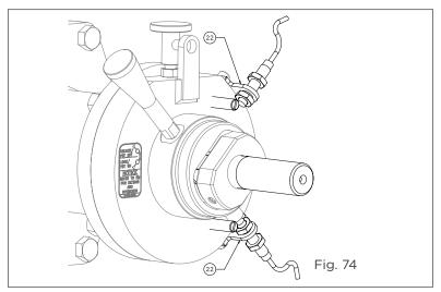
The two indexed positions of the device can be physically locked with a padlock through the indexing plunger, to prevent inadvertent or unauthorized operation of the device.
