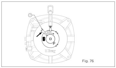
2. Measure the total stroke (S) of the spring rod. First measure the projected length of the spring rod end from the sleeve face. Next, operate the actuator to CCW position and measure the depth of the spring rod face from the sleeve face. Add the two to get the total stroke length.
