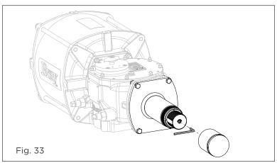
22.2 Installing the Hydraulic Damper on SR actuator
