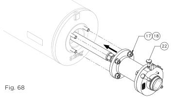
12 Set the PST &LD to "Unlocked" position if not already indexed to this position, by pulling up the index plunger knob(22) and turning the handle (7) upwards till the plunger seats.
