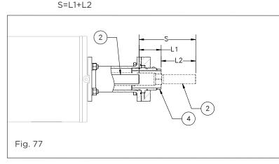
Loosen the locknut (3) by first slackening the set screws (11). Set the distance 'L' between the index sleeve's outer face and the inner face of the locknut per the below table.
