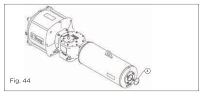
15. Fix back the damper end cover with screws.
