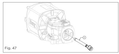
Slacken the set screws (11) and unscrew the lock nut (3) off the extension rod (2). Take care not to drop the plastic buttons (14).
