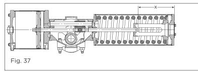
6. This length shall not be less than the solid length of the damper assembly. Use the below guide to check and reset the assembly length "L" of the damper module.
