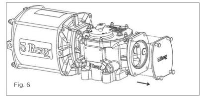
3. Free the Extension Rod from the Jackscrew assembly, apply a drop of medium strength thread lock compound on the extension rod threads and firmly tighten it into the threading in the Guide Block inside the Torque Module. Refer to the piston rod tightening torque table under Section 19.2.
