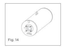
4. Back off the jackscrew fully in the assembly and mount the jackscrew assembly on the spring module end cap thrust base.
