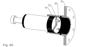
8. Apply a drop of thread lock compound and thread in the studs (8) from the kit into the end cap.
