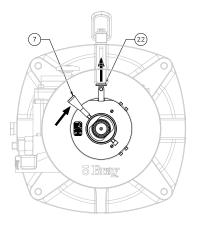
13. Pressurize the adaptor port just enough to rotate the yoke 20 to 30 degrees. Thread in the travel stop bolt to its previously marked position and tighten the seal locknut. Depressurize to get the actuator to its fail-safe position.
