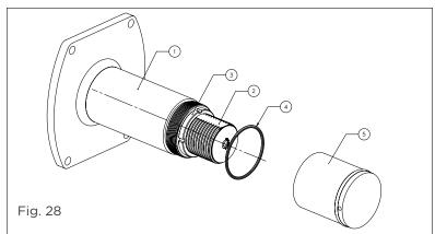
For the end threaded type of dampers, slacken the lock screws (14) and loosen the lock nut (3) to turn the damper (2) in the housing (1).
