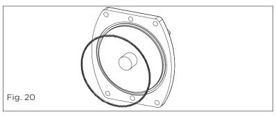
7. Secure the assembly with the mounting bolts, nuts and lock washers from the mounting kit.
