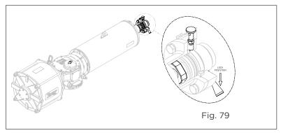
7. Clockwise rotation (to failsafe position of a fail close actuator) of the actuator by depressurizing in this condition will be prevented by the outer face of locknut bearing on the sleeve's inner face, thus mechanically locking the actuator in its CCW end position.
