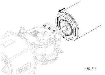
9. Gently push the extended spring rod in and rotate clockwise to engage into the threads in guide block in the torque module. Tighten and torque it to value per below table:
