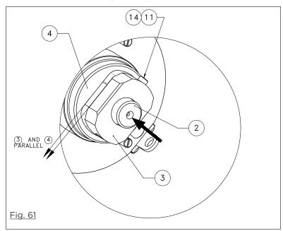
5. With the device in UNLOCKED position, power the actuator to turn counterclockwise. Observe for free movement of the locknut through the sleeve's profile and that the locknut does not rub against the sleeve while moving in. If necessary, reverse the direction and realign the locknut. Fit the tubular cover (6) back on.
