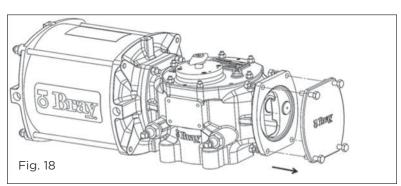
2. Remove the DA end cover from the actuator.
