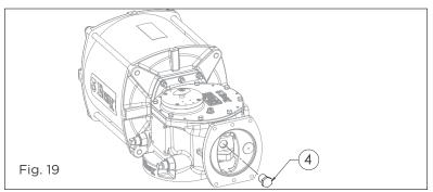
5. Loosen the Lock Nut and back off the Extended Stopper in the assembly.
