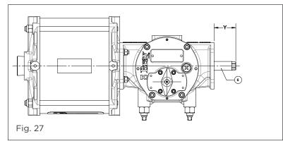
3. For the body threaded type of dampers, unscrew and remove the tubular cover (5). Slacken the ring lock nut (3) and turn the damper unit (2) in the housing (1) to set the length 'L'.
