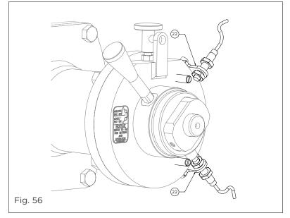
The two indexed positions of the device can be physically locked with a padlock through the indexing plunger knob (23), to prevent inadvertent or unauthorized operation of the device.
