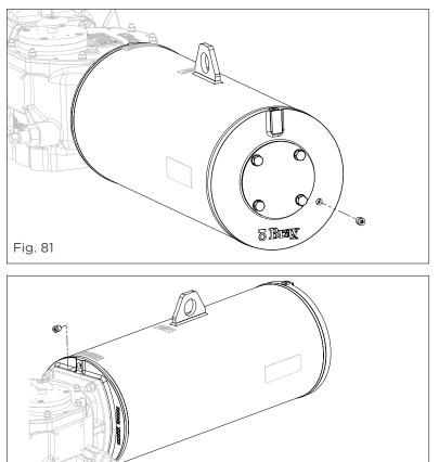
Remove the plugs and connect a pneumatic pipe connector to the port on adaptor, leaving the port on the end cap open.
