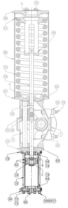
7. Pull out all seals, backup rings and wear rings from the grooves on piston, piston rod, adaptor, end cap and the end cap plug.
