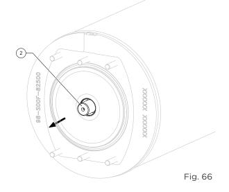
8. Ensure the face sealing O-ring is secure in the spring module adaptor face groove. Lift and mount the spring module back on the actuator, taking care not to damage the rod threads and ensure the spring rod does not slide back out of the module. Tighten the mounting flange stud nuts with spring washers and torque them per table.
