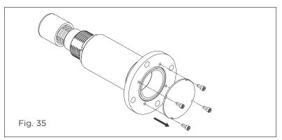
**NOTE:** For all actuator sizes up to 45E3-SR2, the hydraulic dampers have the dampening rate adjustment screw and is located at the rear of the damper unit.
