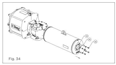
2. Remove Damper end cover from its housing.
