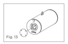
3. Apply a drop of thread lock compound on the mounting stud threads and firmly tighten them into the spring module end cap.
