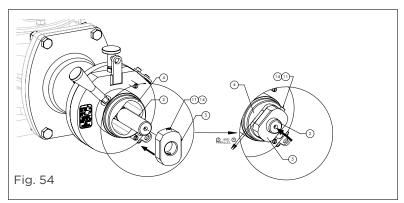
**Note:** Do not turn the nut clockwise to align it with the sleeve, as this could compromise the working clearance required between the locknut's inner face and the sleeve face.
