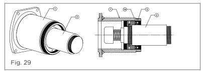
4. Set the length 'L' per the below table and lock the setting with the lock nut (3) or lock screws (14).
