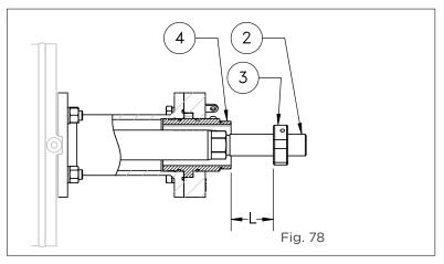
L=S-A, mm S, Stroke Measured, mm
