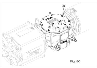
Remove both and fit a pneumatic tube fitting into one of the ports and leave the other one open.
