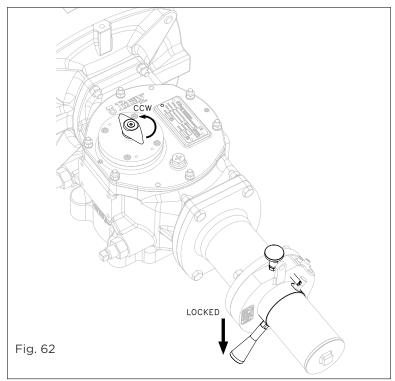
7. Clockwise rotation of the actuator by pressurizing in this condition will be prevented by the outer face of locknut bearing on the sleeve's inner face, thus mechanically locking the actuator in its CCW end position.
