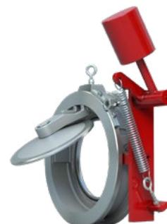
With the external spring it is possible to close the valve before the flow reverses. This reduces or eliminates water-hammer and the associated problems.
