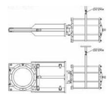
**Figure 5:** Valve with Actuator at 45°
