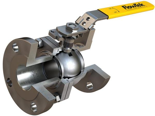
The F15/F30 valve is a two piece, split body construction, allowing ease of maintenance without special tools. These valves feature a "free floating" ball. The ball is not fixed, but is free to move with the line pressure. The spring absorbs this variation while allowing the valve to be installed in any orientation.
