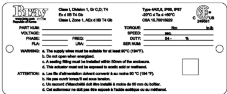
Figure 2: Example ATEX/IECEx certified actuator nameplate.
