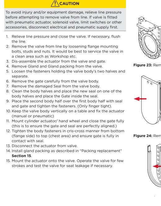
Figure 22: Loosen fasteners and separate valve body halves
