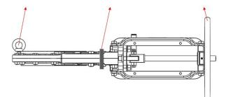
Figure 4: Knife Gate Valve with Handwheel, Horizontal Lifting
