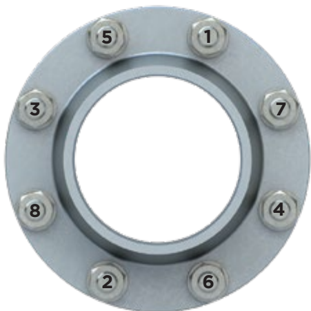
Figure 2 - Flange Bolt Tightening Pattern
