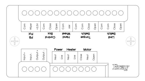
Figure 11: 120VAC / 230VAC Servo NXT terminal labels
