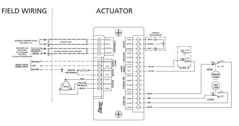
Actuator specific wiring diagram located inside actuator cover.
