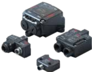
Bray Series 54 Inductive Proximity Sensor SIL 2 Capable
