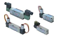
These units can be used with either spring return or double acting actuators where on/off electrical operation is required. Units have 1/4" NPT conduit connections and DIN units have cable gland PG9 connectors, also available with 1/2" NPT conduit adapters.
