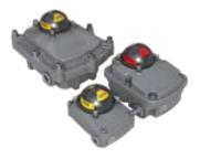
Provide visual and electrical indication of position on any VDI/VDE 3845 compliant quarter-turn rotary actuators. The VSMs can be installed in both perpendicular and parallel orientations without changing brackets. Available as general purpose (Series 5A and 5B) or hazardous locations (Series 5C Explosion Proof, and 5A/B Intrinsically safe).
