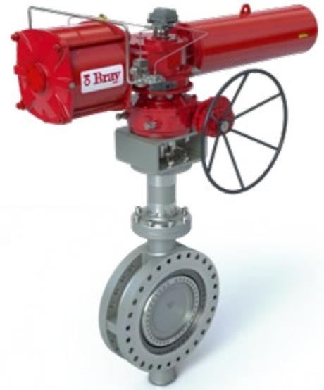
*Tri Lok triple offset butterfly valve; S98 Scotch yoke pneumatic actuator; hydraulic dampener; declutchable override.*
