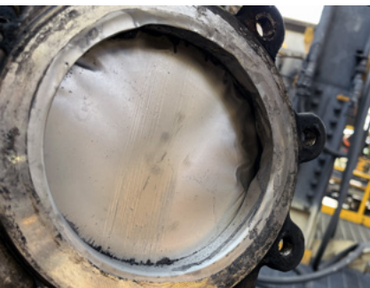
These images show significant signs of damage to existing unidirectional knife gate valves.
