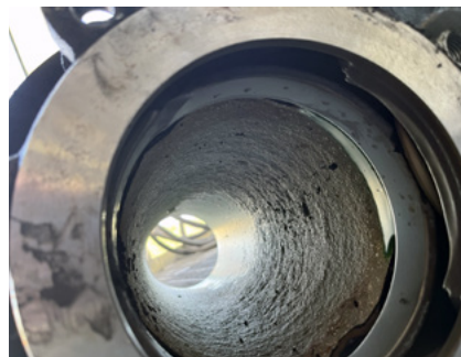
These images show significant signs of damage to existing unidirectional knife gate valves.
