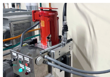
Upper image shows valve and actuator mounted in very tight space. Lower image shows the actuator's hydraulic power unit mounted remotely, due to the space constraints near actuator.
