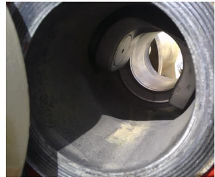
**Inspections showed no erosion to the liner of the Bray evaluation valve.**
