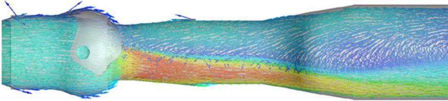
**CFD analysis of the flow highlighted design deficiencies in the failed valves, as well as an optimized solution.**
