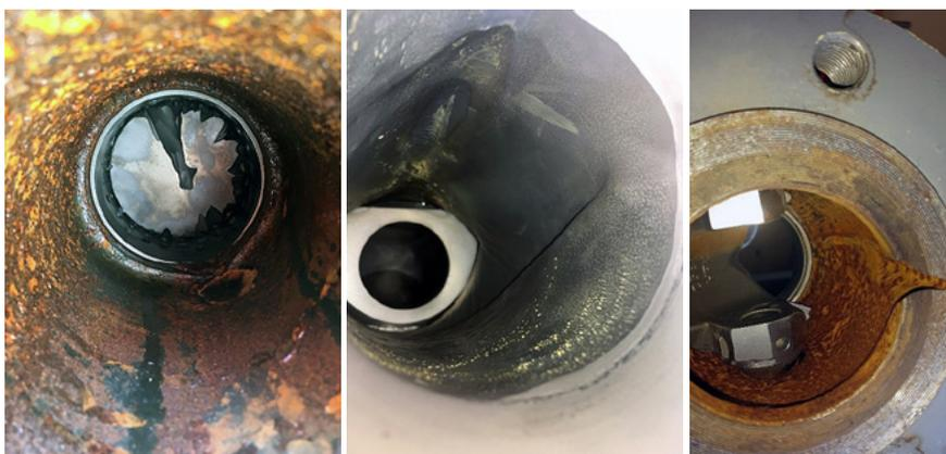
Examples of accelerated erosion in valves that required replacement.
