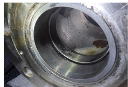
Inspection revealed remnants of the harsh media, but the valve showed no signs of erosion on the ball segment, seat, body walls, or liner.
