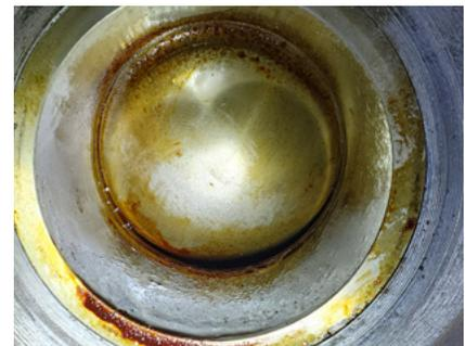
*These images show minimal signs of abrasion to ball segment after 90 days (top) and 180 days (bottom). After each inspection, the valve returned to service.*
