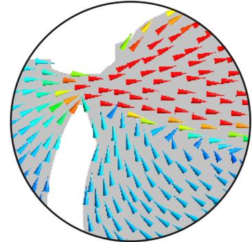
*CFD analysis simulates the flow of the failed valves and proposed solutions.*
