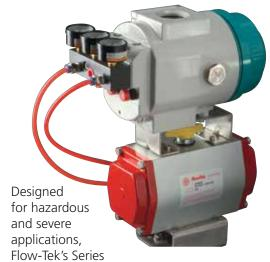
6A explosion proof positioners offer all the features of the waterproof units in a flameproof enclosure. Non-intrinsically safe boards may be placed inside. These rugged, heavy duty units meet EExd IIC T4/T5/T6 specifications. The Automatic Calibration keypad in the explosion proof units are externally mounted and easily accessible. The units can be controlled locally, even during operation, without removing the housing cover. The LCD display is viewed from behind an explosion proof window.
