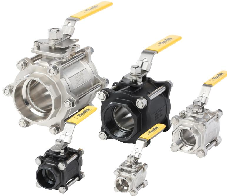
Flow-Tek's Series 5000/6000 ball valves offer the convenience of a three piece body design at an economical price. The 3 Piece design with a swing out center section allows for ease of in-line and out-of-line maintenance. Standard valve bodies are investment cast CF8M Stainless Steel or WCB Carbon Steel. All body castings are marked with a foundry heat number for full traceability.
