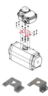
> Stainless steel adjustable bracket for both NAMUR 30 x 80 and 30 x 130 mounting pads (fits all 92/93/98 actuators)
