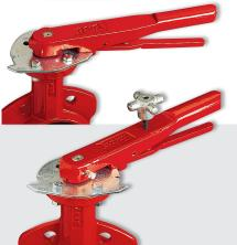
**INFINITE POSITION NOTCH PLATE** for throttling applications, allows for very precise adjustments of valve disc positioning anywhere from 0° to 90°. Positioning is simply a matter of loosening the set knob, moving the handle, then retightening the knob. For resilient seated valves only.
