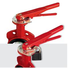
**PADLOCK KIT** allows the customer to lock the valve in the full open or closed position, tamper proofing the valve. By drilling a new hole in the top plate, the handle can be locked in mid travel.
