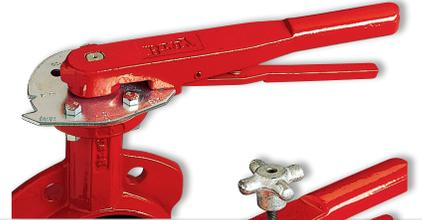
**INFINITE POSITION NOTCH PLATE** for throttling applications, allows for very precise adjustments of valve disc positioning anywhere from 0° to 90°. Positioning is simply a matter of loosening the set knob, moving the handle, then retightening the knob. For resilient seated valves only.
