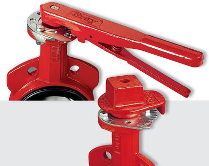
**2" SQUARE NUT** is used where the valve is buried under the surface. To rotate valve disc position, the nut is reached with a T-handle wrench.
