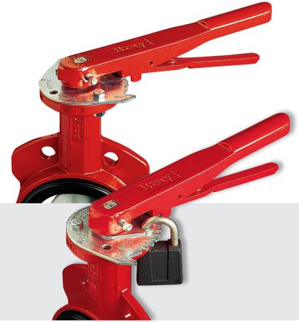
**PADLOCK KIT** allows the customer to lock the valve in the full open or closed position, tamper proofing the valve. By drilling a new hole in the top plate, the handle can be locked in mid travel.
