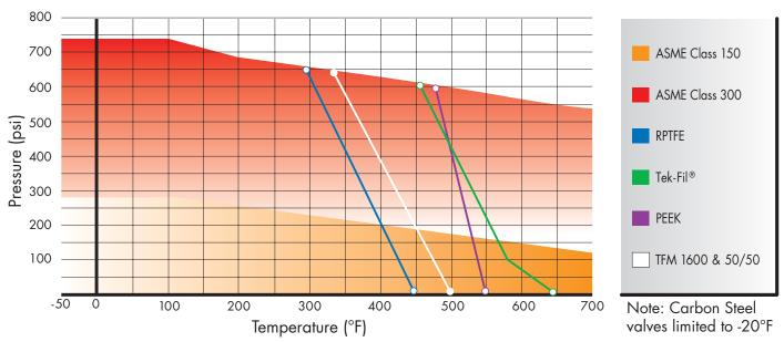
Carbon Steel valves limited to -20°F
