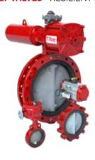
Bray's resilient seated butterfly valve line has been an industry leader for over 30 years. Tongue and groove seat design, double-D shaft to disc connection, and Nylon 11 disc coating are all best in class features which provide a long lasting and quality product.
