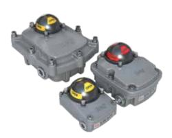
Series 5A, 5B and 5C Valve Status Monitors (VSM) provide visual and electrical indication of position on any VDI/VDE 3845 compliant quarter-turn rotary actuators. The VSMs can be installed in both perpendicular and parallel orientations without changing brackets. Available as general purpose (Series 5A and 5B) or hazardous locations (Series 5C Explosion Proof, and 5A/B Intrinsically safe).
