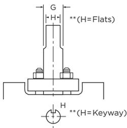
\*\* Keyway is applicable on valve sizes 14"- 54" Class 150 valve sizes 10"- 48" Class 300 valve sizes 8"- 30" Class 600
