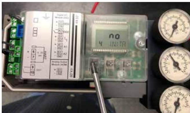
3.2.6 Hold down the Up Button
