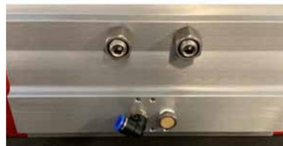
Professionally fabricate and connect air line between the positioner and actuator. The tubing must not contact the actuator as this may lead to tube wear/leakage in a vibrating application.
