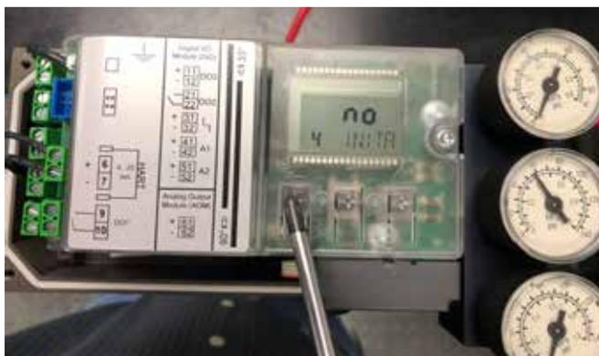
3.1.10 Hold down the Up Button
