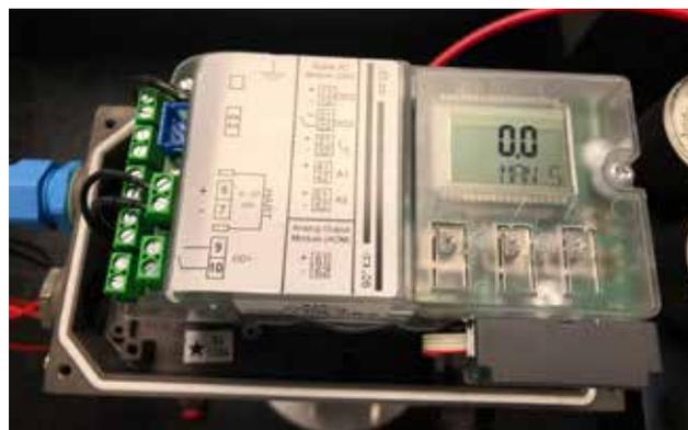
3.2.9 Use the ▽ or ▲ buttons to manually close or open the valve to ensure that the desired travel limits are being attained.
