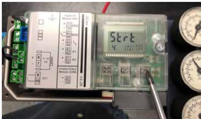
3.1.11 **Note:** If an error is displayed on your positioner during Run 2, the lower tolerance (down tolerance) of the adjustment wheel has been exceeded. (If no errors are displayed, skip ahead to step 3.1.12.)
