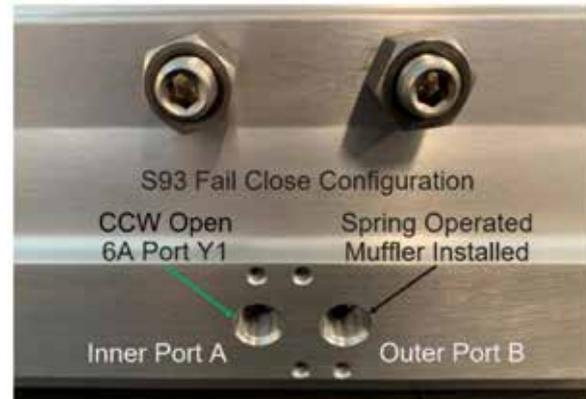
Only the inner port A will be connected to the 6A positioner at port Y1. The piston rack to pinion orientation determines the spring fail position, see S92/S93 IOM for details.
