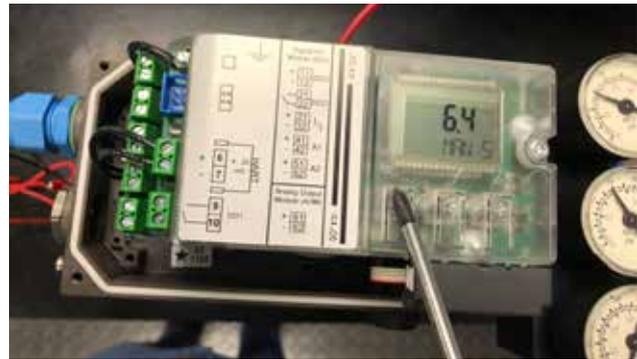
3.2.11 While in ‘AUTO’ mode, test the responsiveness of the device by varying the command signal from 4 mA to 20 mA.
