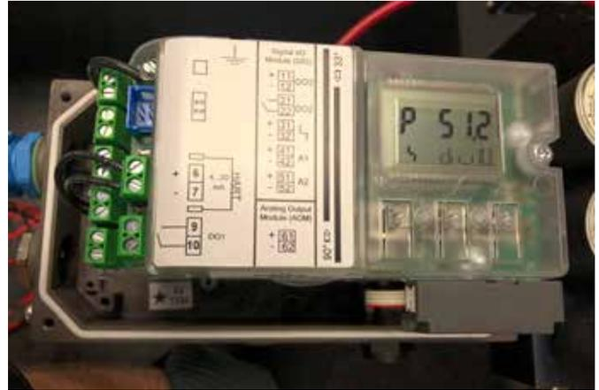
3.1.11.1 Adjust the gray friction clutch adjustment wheel until the screen displays a “6” in the top right hand corner.
