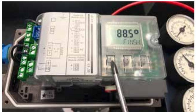
3.1.13 Press the Menu Button
