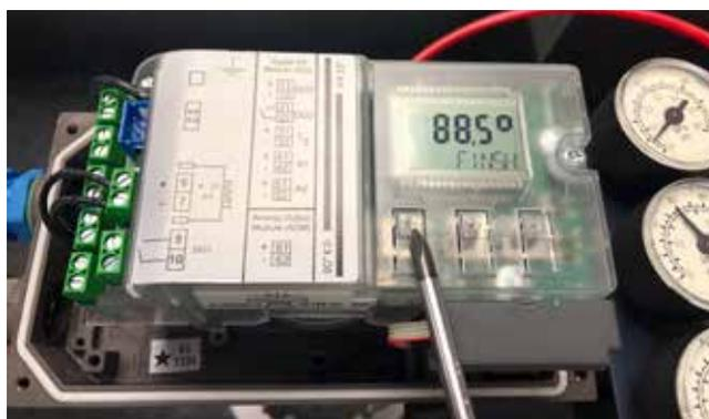
3.2.8 Press the Menu Button
