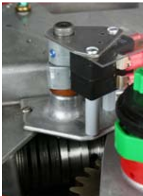
OPTIONAL TORQUE LIMITING SWITCH SYSTEM
